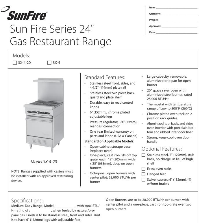
Oven: Oven door is to be one piece. Aluminized top, back, and sides oven interior with porcelain bottom and ribbed inter door liner. Thermal protectors keep the oven door handle cool to the touch. Oven to come with a thermostat having temperature range from Low to 500°F, (260°C). Oven interior is to have one chrome plated oven rack and two-position rack guides.
